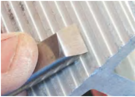
▲ Pic.4 Here I have ground off the heel of the skew; it negates the fact that the tool is hollow ground, otherwise it could mark the wood. The angle across the top is around 15°
